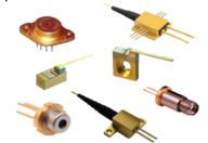
The LDX-3415-808 is a high power, infrared laser diode chip. The InAlGaAs laser design offers low divergence, high brightness, and proven reliability. Applications include solid-state laser pumping, materials processing, and medical applications.
