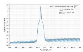
Typical spectrum of 0405 nm diode laser. Measured with 10 pm resolution.
