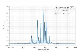
Typical spectrum of 0445 nm diode laser. Measured with  $10\ pm$  resolution.
