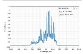
Typical spectrum of 0515 nm diode laser. Measured with 20 pm resolution.
