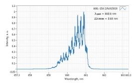
Typical spectrum of 0660 nm diode laser. Measured with 20 pm resolution.
