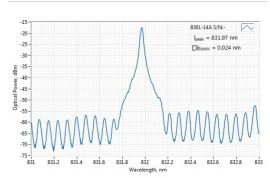
Typical spectrum of 0830 nm diode laser. Measured with 20 pm resolution.
