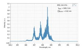
Typical spectrum of 0850 nm diode laser. Measured with 20 pm resolution.
