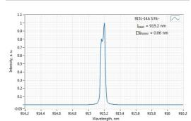
Typical spectrum of 0915 nm diode laser. Measured with 20 pm resolution.
