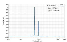
Typical spectrum of 0975 nm diode laser. Measured with 20 pm resolution.  $\,$
