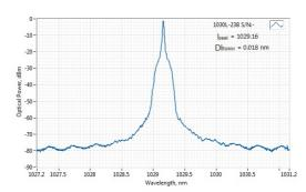
Typical spectrum of 1030 nm DPSS laser. Measured with 20  $\ensuremath{\mathsf{pm}}$  resolution.
