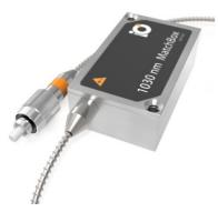
1029 nm laser module is a DPSS laser with Yb:YAG gain medium and high power pump. The SLM version of this laser is used for inspection of optical components at a wavelength, which is popular in high power fiber lasers and ultrashort pulse DPSS lasers. Beam if this 1029 nm SLM laser module is delivered through a multimode fiber.
