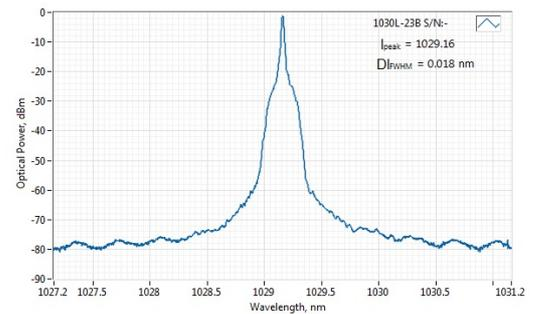
Typical spectrum of 1030 nm DPSS laser. Measured with 20 pm resolution.
