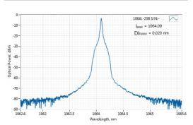
Typical spectrum of 1064 nm DPSS laser. Measured with 20 pm resolution.
