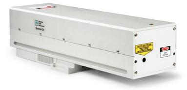
Quantas Q2 models employ MOPA (Master Oscillator / Power Amplifier) architecture in order to produce high pulse energies while maintaining low divergence output. Two models are available, offering 50 mJ @ 20 Hz or 70 mJ @ 10 Hz pulse energies.
