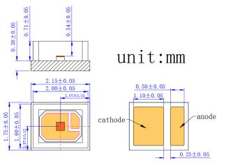
VD-0850P-010W-3A-3A0 (Channel array 1x1, Substrate CuAg, Package 2016)
