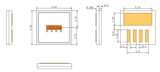
VD-0850P-050W -10-3A0 (Channel array 1x8, Substrate Cu/Ag, Package 1x8)
