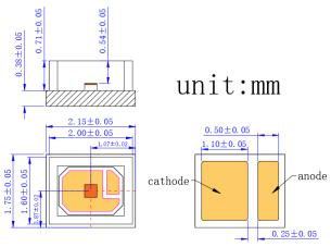
VD-0850P-050W-3A-3A0 (Channel array 1x1, Substrate Cu/Ag, Package 2016)
