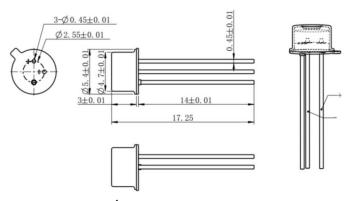
VD-0850P-050W -1N-3A0 (Channel array 1x4, Substrate AIN, Package 1x4)
