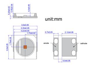
VD-0850P-400M-3E-2A0 (substrate CuAg Package 7060) ), unit:mm
