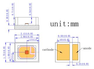
VD-0850P-700M-1C-2A0 (substrate AIN 3535 packaging), unit:mm
