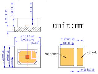
VD-0940P-010W-3A-3A0 (Channel array 1X1, Substrate CuAg, Package 2016)
